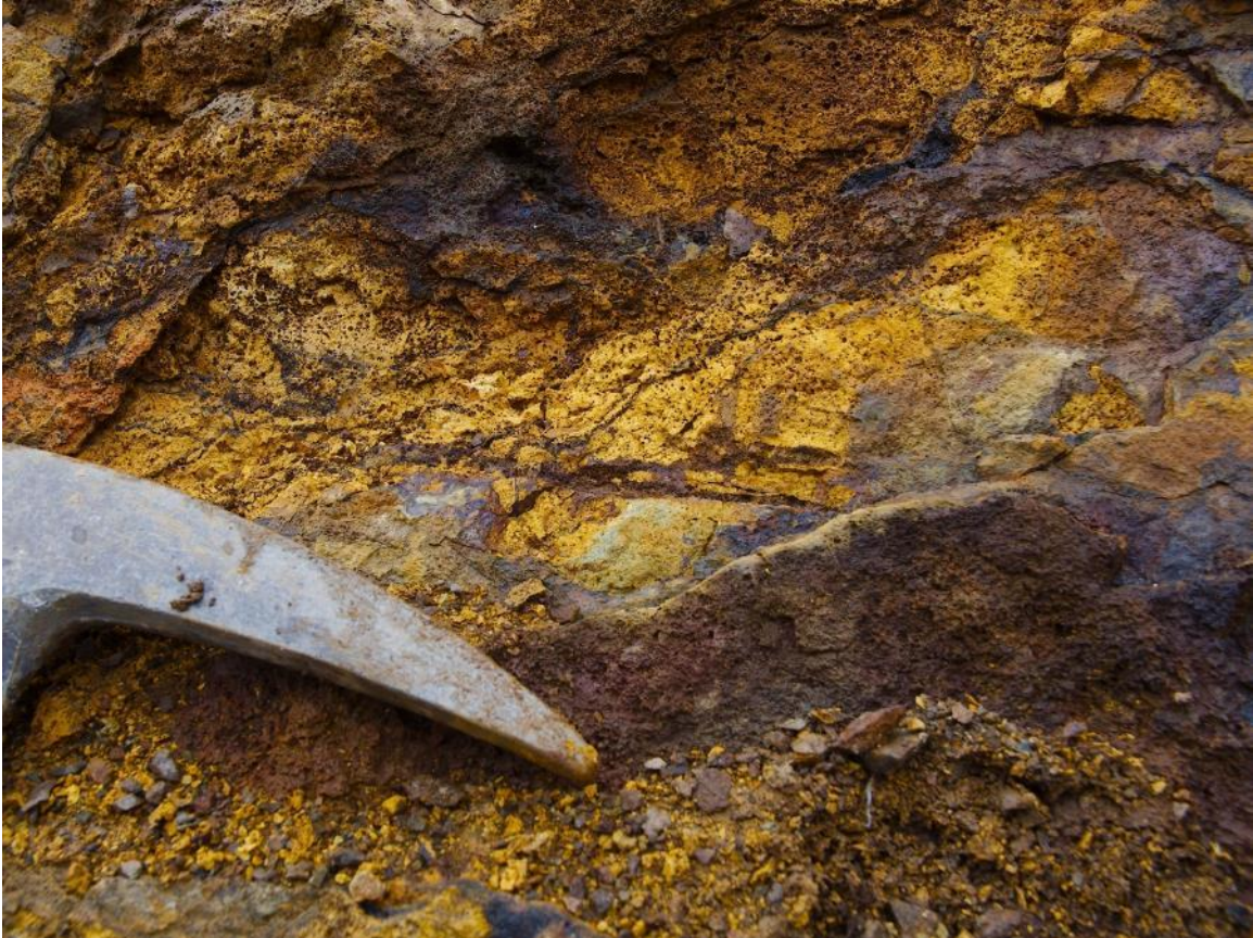
Figure 5 - Typical appearance of the strongly pyritic and supergene oxidized rocks located between members of the potassic altered dyke swarm.
