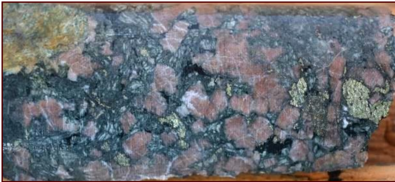
Above: Potassic alteration and copper mineralization intersected in drill hole DK-2023-003 Right: Soil geochemistry, top copper in soils, middle gold in soils, bottom molybdenum in soils
